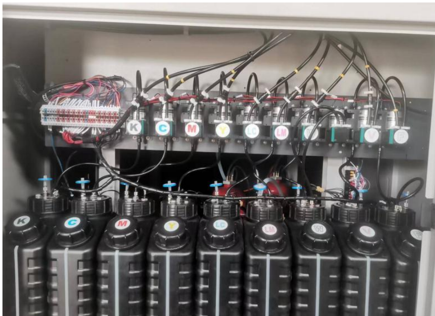
Fig. 95: Location plan of main ink tanks
