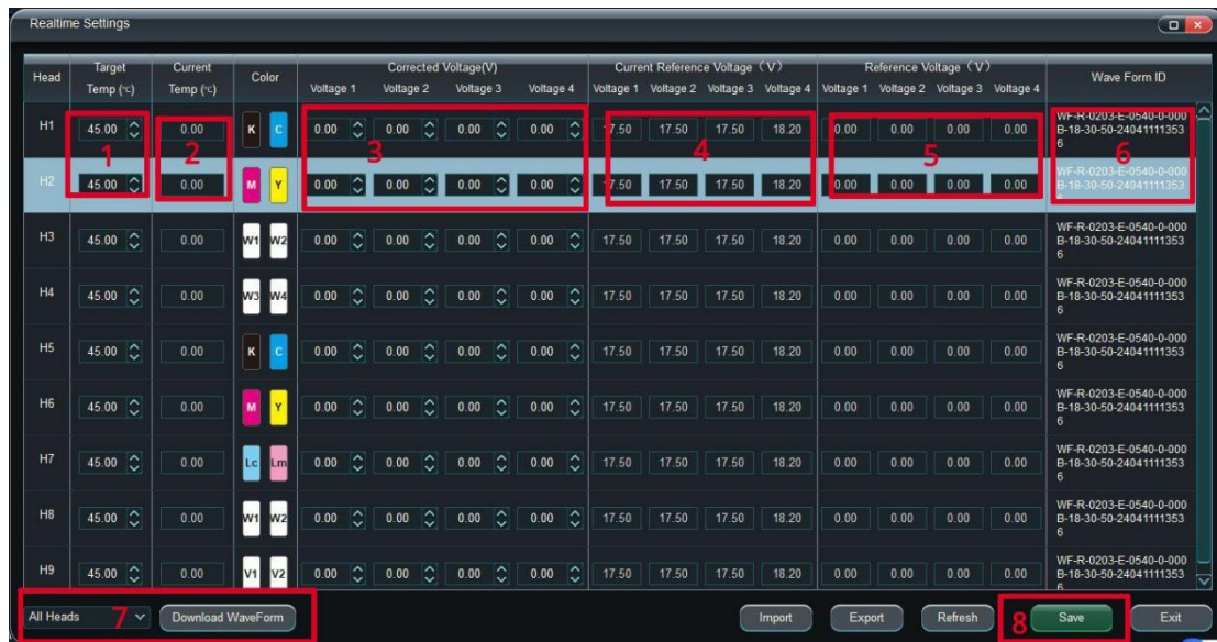
Fig.111: Temperature settings of the print head
