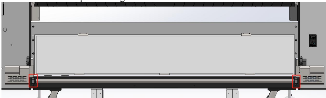
Fig. 31: Diagram of the installation locations and finished installation of the transition roller components
