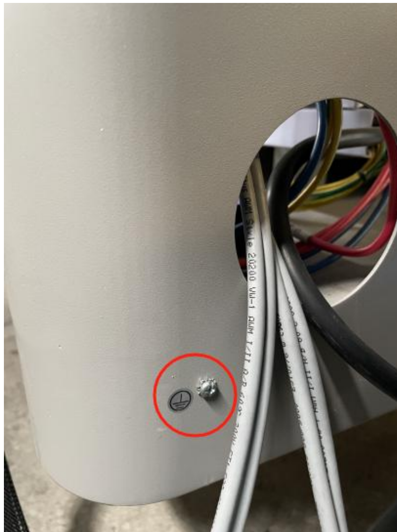
Fig. 37: Diagram of grounding position of UV hybrid printer
