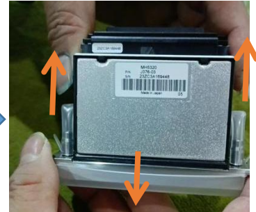
Remove the plug tube of the ink inlet and remove the protective cover for the nozzle surface.
