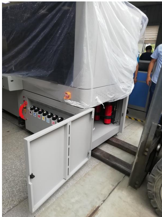
Fig. 16: Transportation of the machine with fork under both ends
